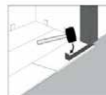
2. Use mallet and pull bar to tap in and lock short side of board.
