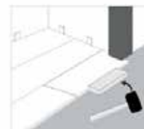
1. Undercut door jamb to allow board to slide freely under. Tap long side of board using mallet and tapping block to lock in long side.
