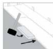
5. Use mallet and tapping block or scrap piece of board with matching undamaged click tongue to tap long side of board to ensure a tight fit. Tapping block should be min. 250mm long. Any gapping will compromise the locking system.
