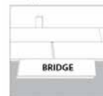
6. Attach a scrap piece of board to bridge gap between ends of planks.
